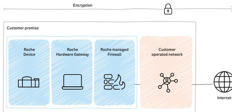
The Roche managed firewall is located within the customer laboratory network to protect Roche devices from cyber-security threats. It is a stateful firewall manufactured by the leading firewall company - Fortinet, with a custom configuration for Roche medical devices.
